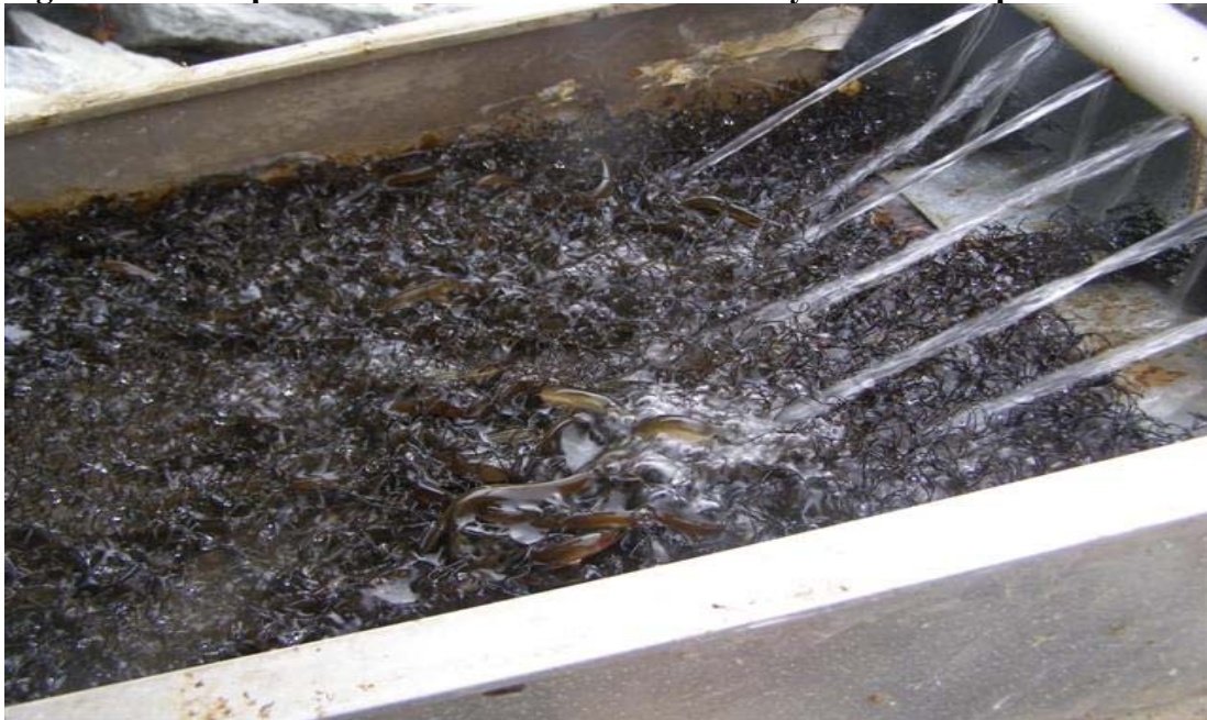
Figure 2. Eel trap constructed of industrial cable tray and landscape fabric.
